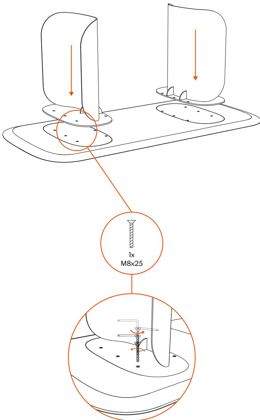
Avvitare la piastra al piano (sottosopra). | Screw the metal plate to the top (upside-down).
