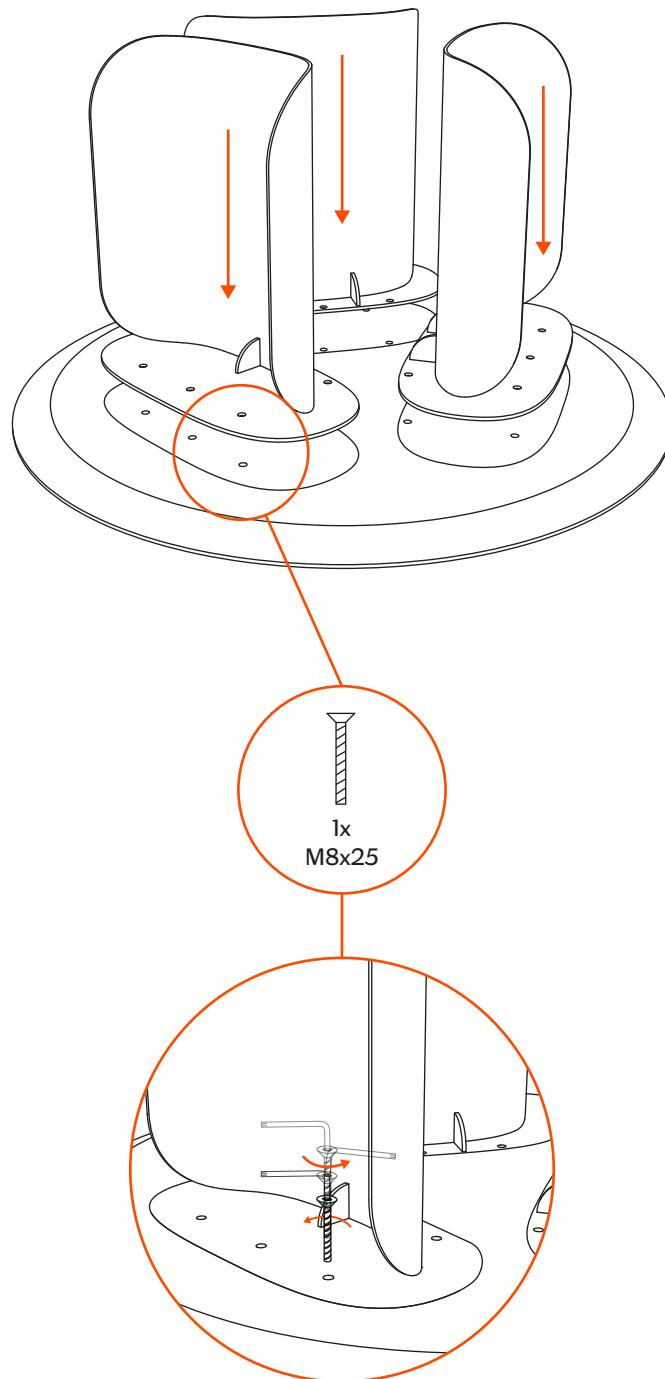
Avvitare la piastra al piano (sottosopra). | Screw the metal plate to the top (upside-down).
